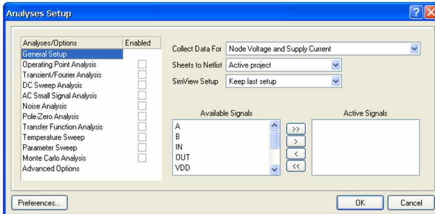
All the simulation options are set up here, including the analyses types you want to include in the simulation, the scope of the simulation (sheets to netlist) and the signals to be automatically displayed when the simulation is complete (active signals). These options are stored in the project file (when saved) and will be used in the creation of a SPICE netlist (\* .nssx) which is used when the simulation is run.
