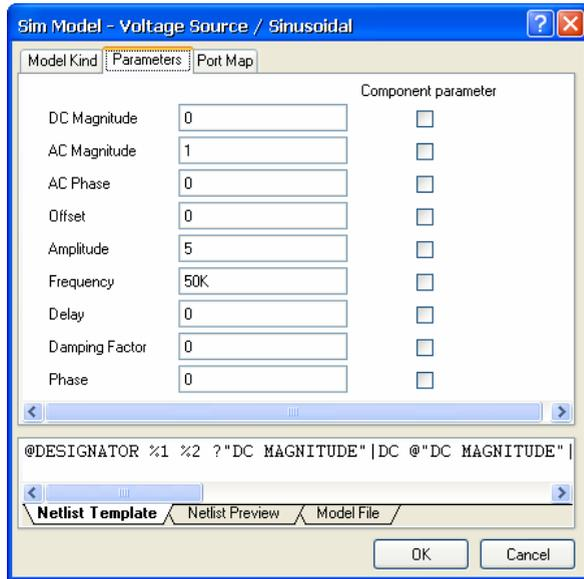
Click **OK** until the dialogs are closed and click to place this voltage source on the schematic. Right-click or press **ESC** to exit placement mode.
