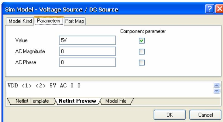
Click **OK** until the dialogs are closed. Click to place this voltage source on the schematic. Right-click or press **ESC** to exit placement mode.
