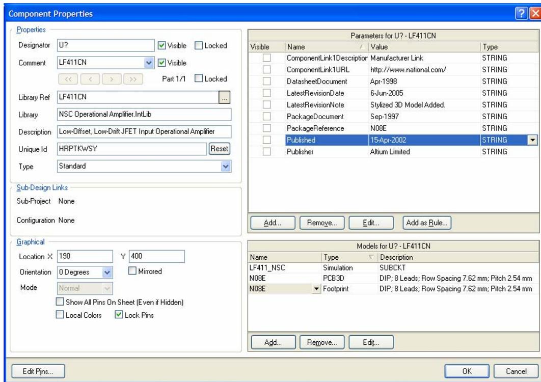
5. In the **Properties** section of the dialog, set the value for the first component designator by typing U1 in the **Designator** field.
