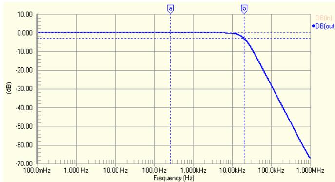
4. Read off the X value of cursor B in the Measurement Cursors section of the **Sim Data** panel and you will find the 3dB point = 20kHz.
