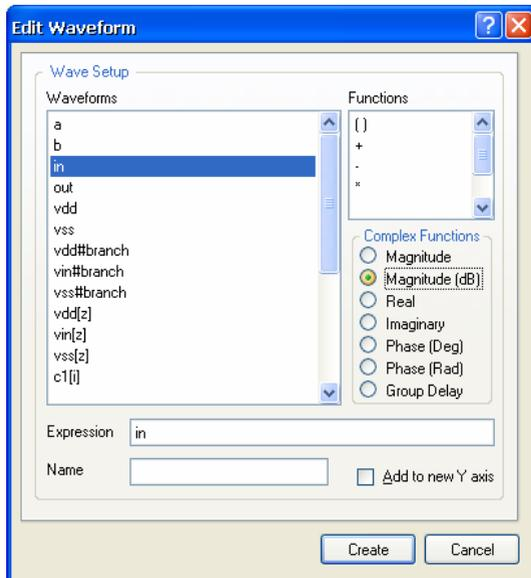
3. Select the function from the Complex Functions list, i.e. Magnitude (dB). Click on **Create** to see the waveform `dB(net_name)`, i.e. `dB(in)`, on the plot.
